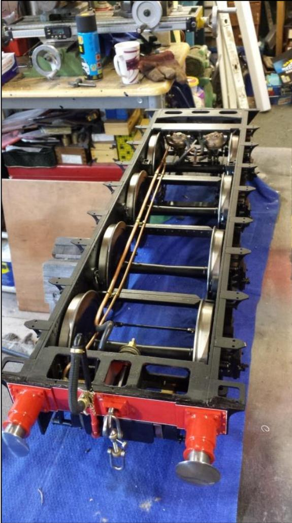
The chassis is fully painted although has a few bits of the lining to finish, most of it is there. The tender as with the locomotive is vacuum braked, both having two vacuum cylinders, these are all finished and tested, it's a shame that you can't add video to a newsletter...☺
